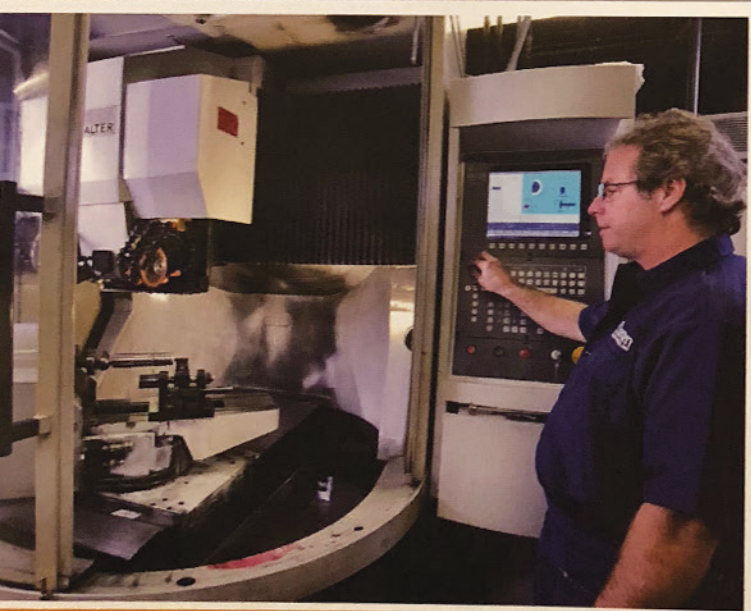
Other applications require special grinding equipment like this Walter Helitronic Power Production Tool & Cutter grinder for highly accurate and complex pieces.
