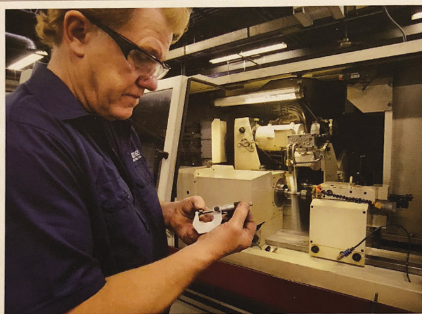
Every Damen Carbide part is completely inspected – manually on small runs and Zeiss CMMs for longer run jobs.
