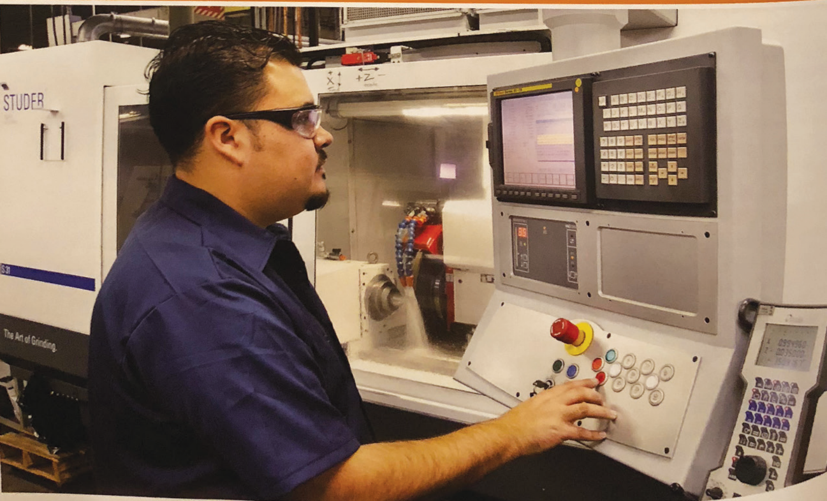
The Studer S31 is designed for the grinding of workpieces in individual as well as small and large series production operations. It can be automated and is — thanks to its universality — especially suitable for use in the tooling and aerospace sectors, for example. The machine features a revolving wheelhead that can be swiveled manually or automatically, a high-resolution B-axis, a frequency-controlled motor grinding spindle for ID and OD grinding, and a C-axis for the workhead for form and thread grinding.
